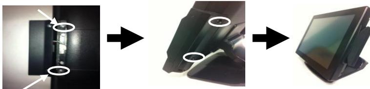
**Step A:** Remove these 2 screws to remove the side mount cover on the back of the right side mount upgrade kit.
