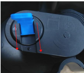
⑤ Load new receipt roll, then insert Receipt paper under the slot of winding Bobbin
